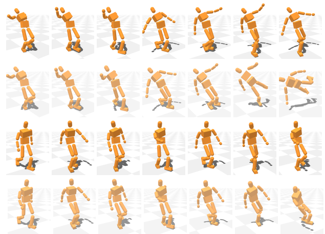
Figure 8: Comparison of the parameterized controller (row 1, 3) and the baseline controller (row 2, 4). Row 1, 2: Simulation of the reference motion for \mathbf{P} = (0.05, -0.05, -0.15) . Row 3, 4: Simulation of the reference motion for \mathbf{P} = (0.05, -0.05, 0.05) .
