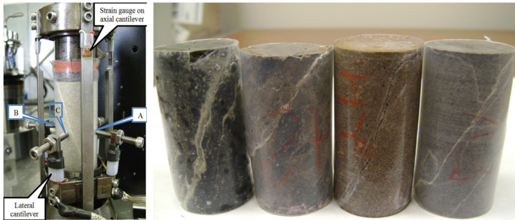
Fig. 14. (a) Sample assembly for triaxial testing (left); and (b) four samples after testing (left to right: N1-4013-1H, N1-4348-2H, N2-4219-2H, Oxy-4394.5-4396-5 V). (b) Shows that texture and fabric of each sample has influenced rock failure. Note different failure configurations from left to right: fracture along a healed fracture; failure through clay-rich weak zone propagating around a strong inclusion; highly localized shear plane; and failure on multiple healed fractures with predominant motion along a major fracture.
