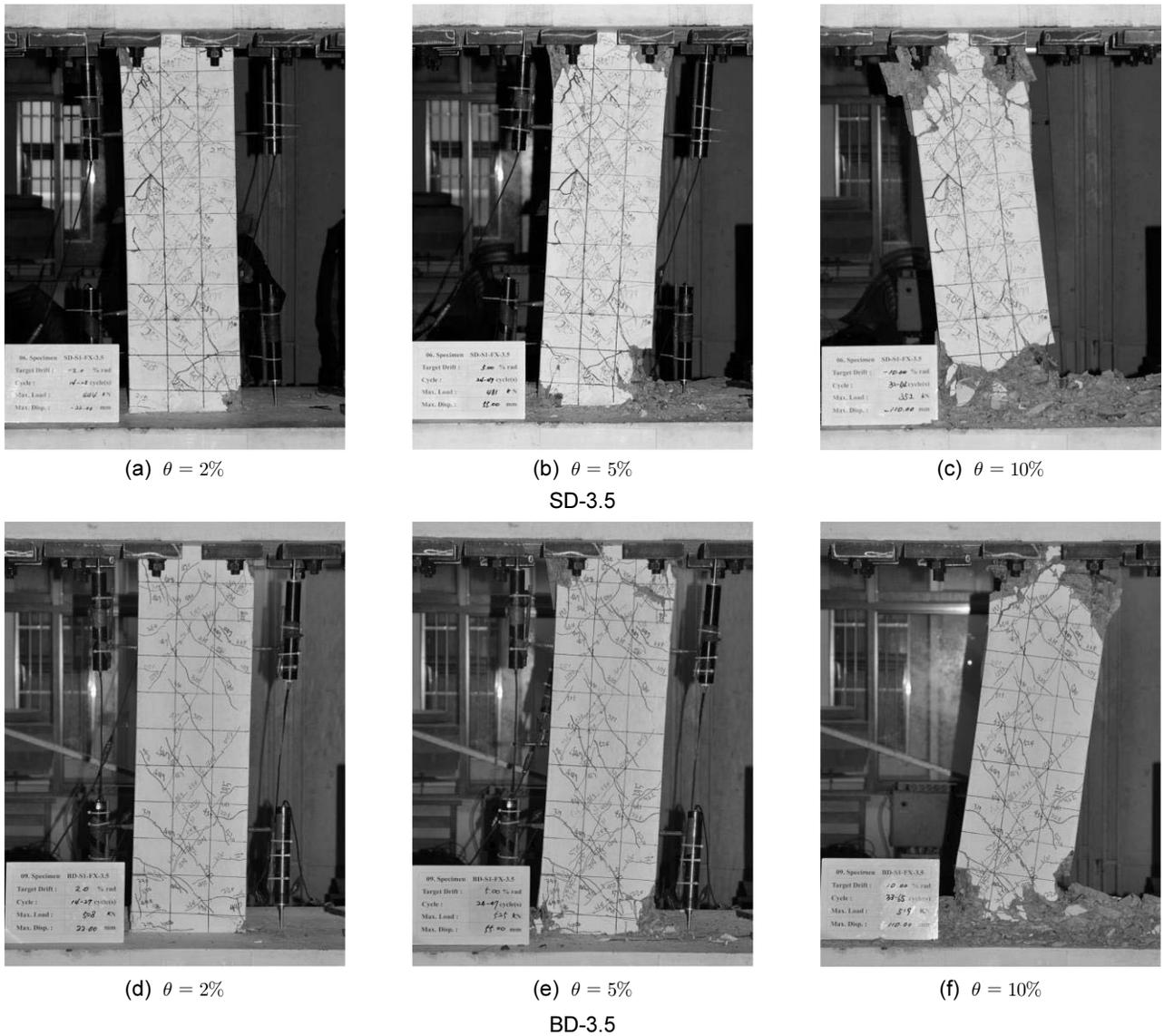
**Fig. 8** Crack progression
