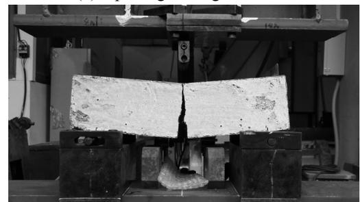
(c) Flexural Strength Test
