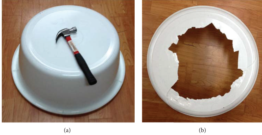
FIGURE 21: Arbitrary target area. (a) A hole creation by using hammer and (b) the created hole.
