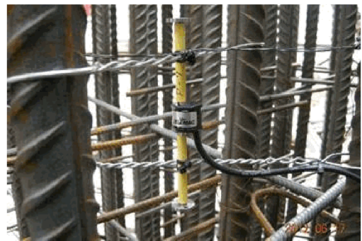
Fig. 2 Vibrating wire strain gauge
