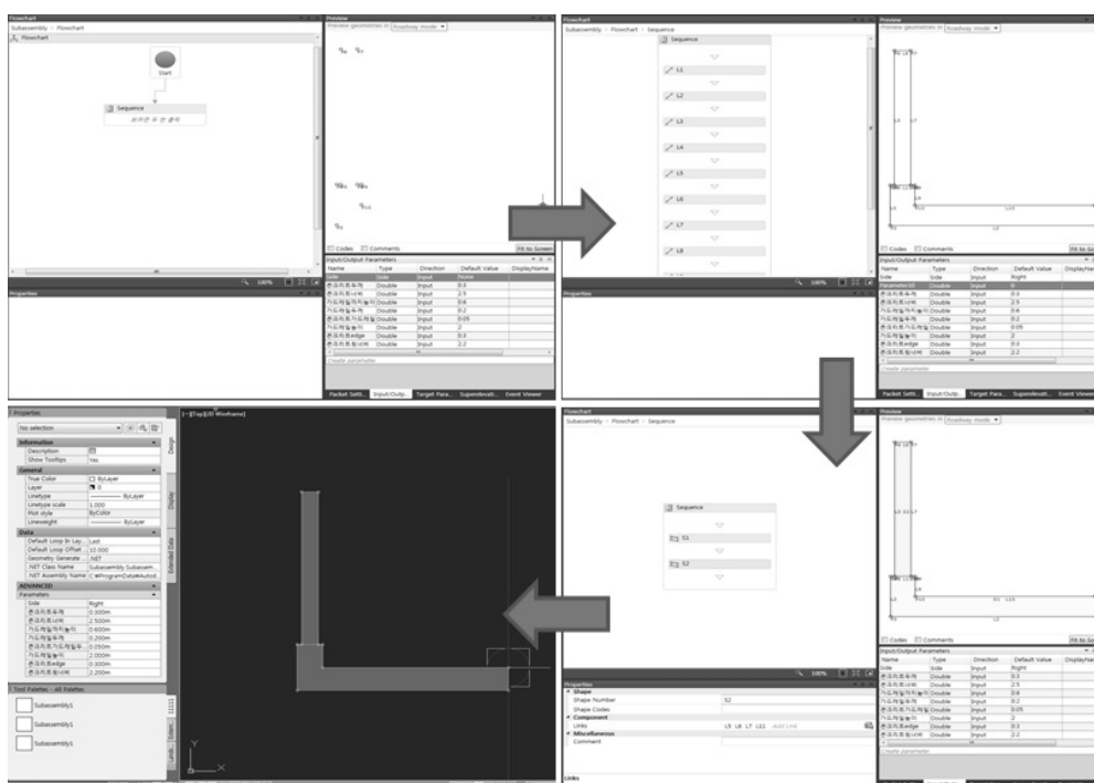
Fig. 4. Sub-assembly Production Process of Using "Autodesk Sub-Assembly Composer"
