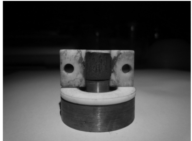
Fig. 2. Photograph of \text{TiH}_2 specimen, frozen at -25^\circ\text{C} in Teflon container with Cu bottom plate.
