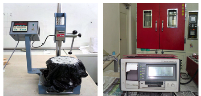
Fig. 3 Measurement of the penetration resistance and the length change
