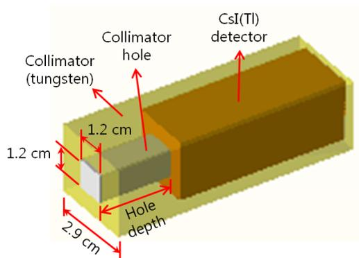
**Figure 1.** Geometry of collimator.
