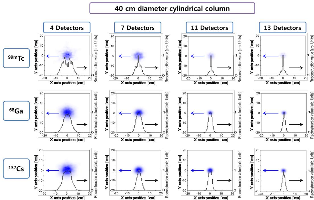
**Figure 3.** Reconstructed images (left hand side vertical axis and horizontal axis) and corresponding image profiles at  $y=0$  (right hand side vertical axis and horizontal axis) for the 40 cm diameter column.
