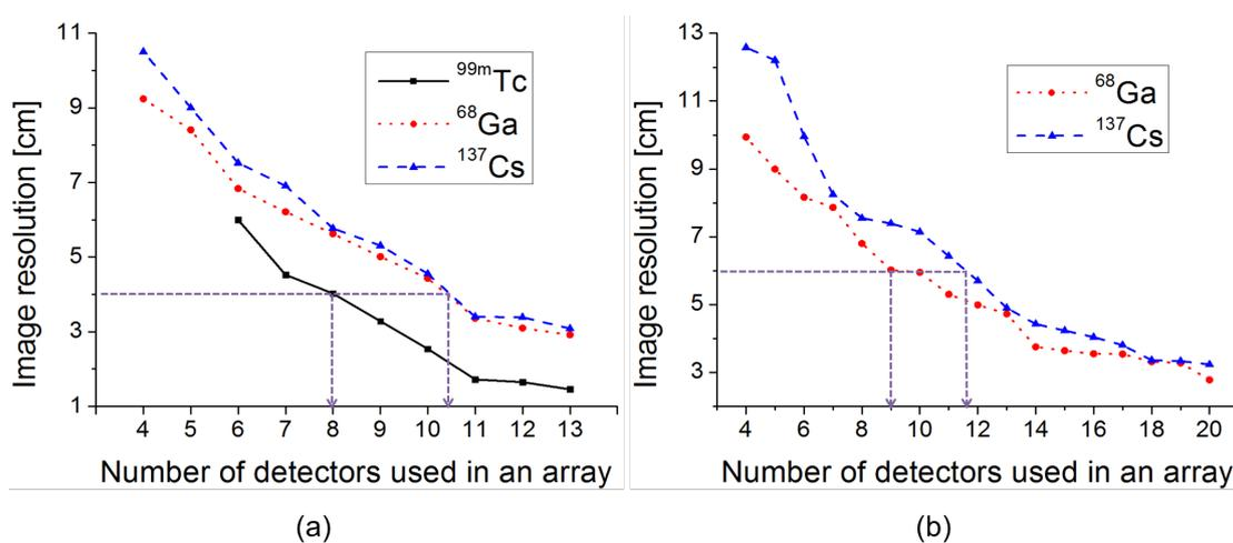
**Figure 5.** Calculated FWHM of the profile as a function of the number of detectors for the 40 cm diameter (a) and 60 cm diameter (b) columns.
