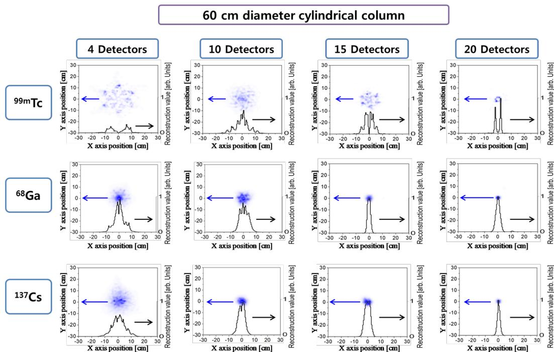
**Figure 4.** Reconstructed images (left hand side vertical axis and horizontal axis) and corresponding image profiles at  $y=0$  (right hand side vertical axis and horizontal axis) for the 60 cm diameter column.
