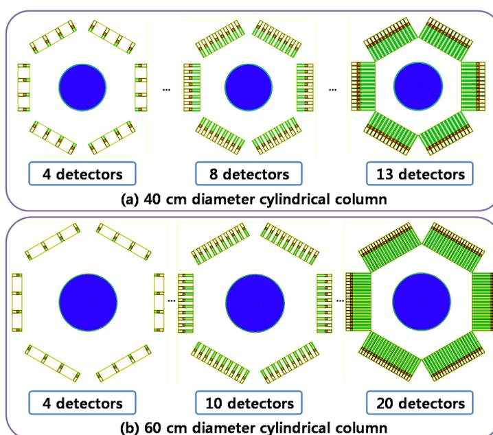
**Figure 2.** Schematic diagrams of (a) 4, 8, and 13 detectors for the 40 cm diameter column and (b) 4, 10, and 20 detectors for the 60 cm diameter column.
