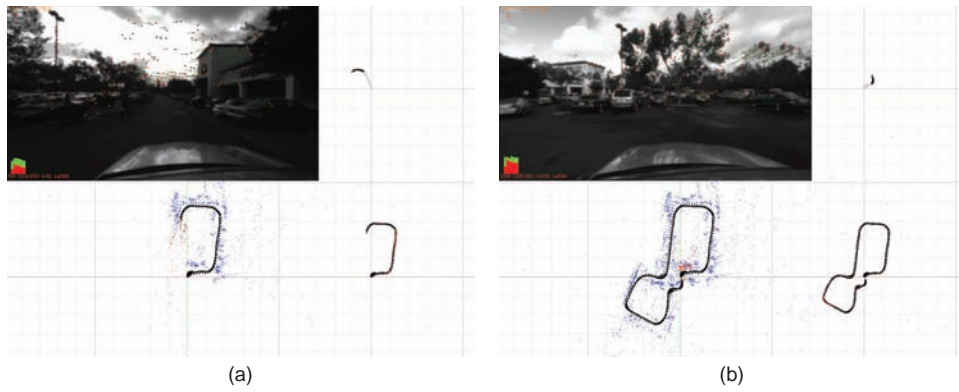
Fig. 11. The snapshots from a car sequence ‘Parking Lot’. (a) The features from moving objects (a pedestrian and a truck) are regarded as outliers in the RANSAC process, and not included in the map. (b) After a loop in a parking lot, the car’s location is quite accurately estimated even though the loop closure from feature matches did not occur.
