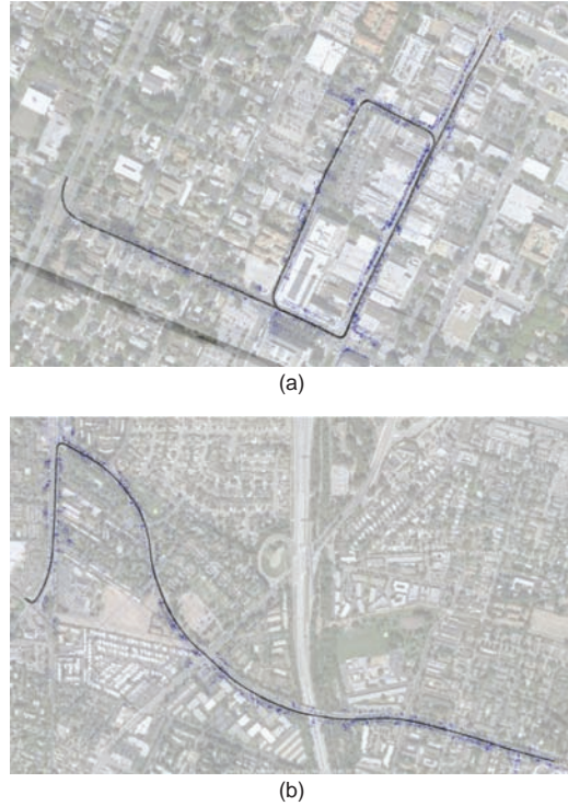
Fig. 12. The environment maps are overlaid on top of the aerial photos from Google Earth. The global location, rotation, and scale of the map plots are manually adjusted to the aerial photos. The results show very high accuracy in spite of the long distances travelled. (a) Castro St. (b) Middlefield Rd.
