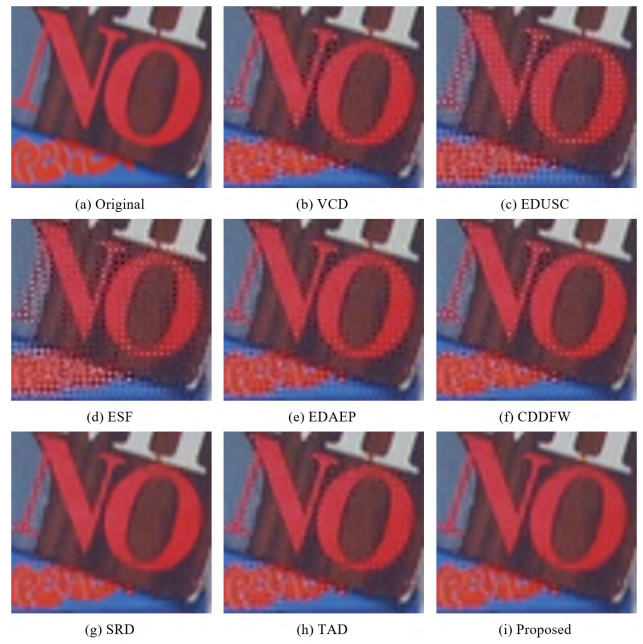
FIGURE 18. Comparison of (a) original image and result of the (b) VCD, (c) EDUSC, (d) ESF, (e) EDAEP, (f) CDDFW, (g) SRD, (h) TAD, and (i) Proposed methods (LC #1).
