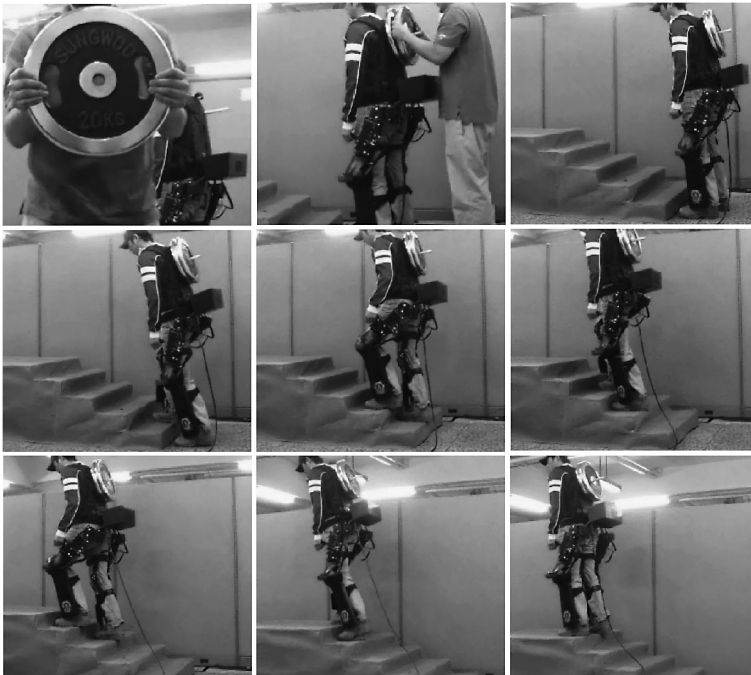
Figure 12. Performance test of the developed system (step walking while carrying a weight of 40 kg).
