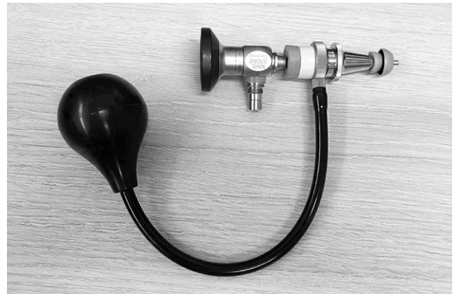
Fig. 1. Pneumatic adaptor with rubber bulb connected to an endoscope.
