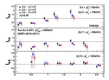
FIG. 6.  $I_{AA}$  as a function of  $\xi$  for direct photon  $p_T^{\gamma}$  of (a) 5–7, (b) 7–9, and (c) 9–12 GeV/c. Three away-side integration ranges are chosen to calculate the per-trigger yield and the corresponding  $I_{AA}$ :  $|\Delta\phi-\pi|<\pi/2$  (closed [black] circles),  $|\Delta\phi-\pi|<\pi/3$  (closed [blue] squares), and  $|\Delta\phi-\pi|<\pi/6$  (closed [red] triangles).
