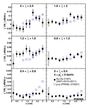
FIG. 2. Per-trigger yield of hadrons associated with direct photons in Au + Au collisions (closed [black] circles) for direct photon  $p_T$  5–9 GeV/c, compared with p+p baseline (open [blue] squares), in various  $\xi$  bins.
