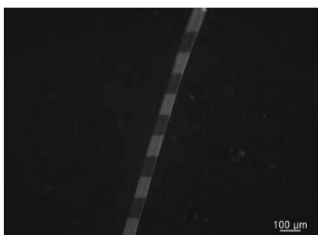
Figure 3. Patterned fluorescence images obtained from photomasked UV irradiation (254 nm, 1 mW/cm 2 , 2 min) followed by PEB (100 °C, 1 min) of a t -BocQ containing single electrospun fiber.
