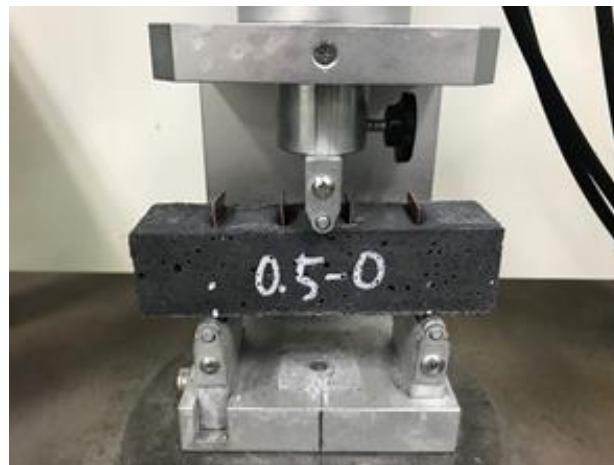
Figure 7. Induction of flexural crack at the mid-span of the specimen.
