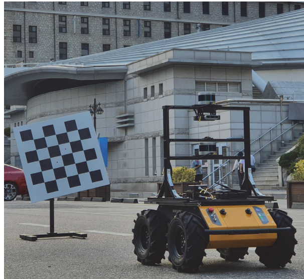
Photo. 1 Checker-board based camera-LiDAR calibration
