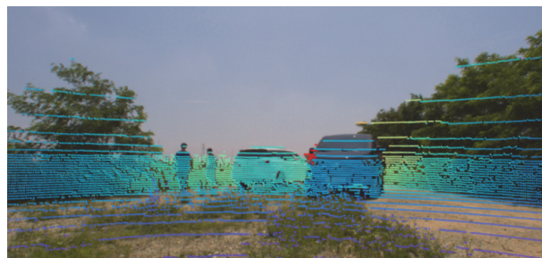
Photo. 3 Projection of point clouds to the image plane after camera-LiDAR calibration
