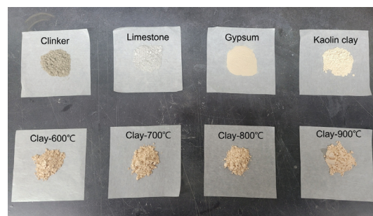
Fig. 1. Raw materials of control and LC 3
