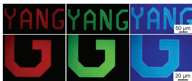
Figure 2. Patterned fluorescence images of a spin-coated film on a glass substrate containing t -Boc-DDPD after photomasked irradiation with 254 nm (1 mW/cm ^2 ) UV irradiation for 3 min and PEB (100 ^{\circ} C, 1 min) process. Excitation wavelength: red (546 nm), green (488 nm), and blue (357 nm), Exposure time: red (1/9 s), green (1/9 s), and blue (1/120 s).
