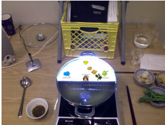
Fig. 1. Inductive hot-plate and the NetPot system of projected remote diner actions, chopstick tracking cameras and Skype audio teleconferencing
