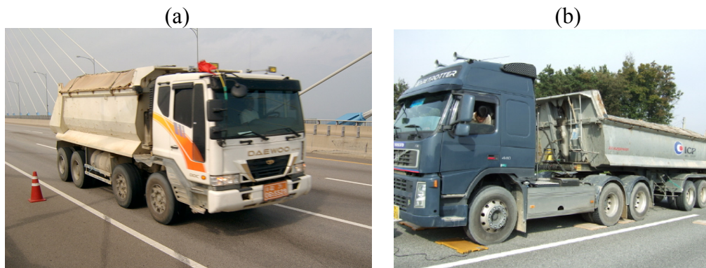
Figure 5. (a) Experimental test on Seohae Bridge. (b) Static weighing of test trucks for Geumdang Bridge.
