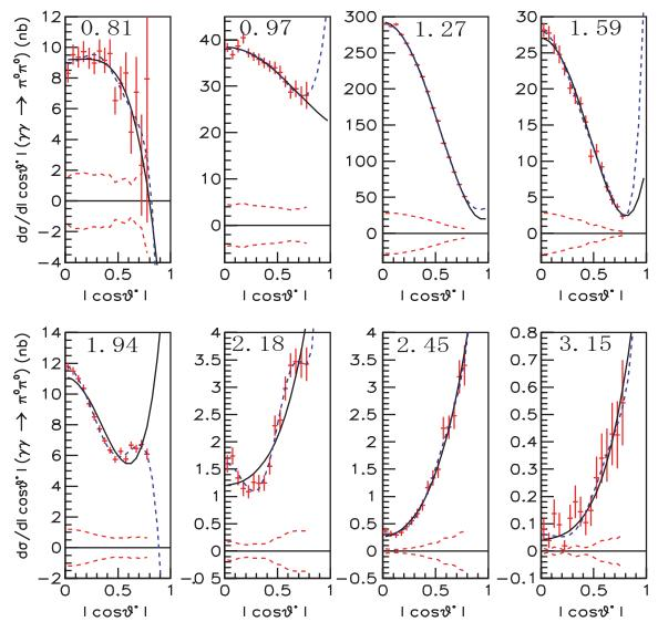
FIG. 7 (color). Differential cross sections for the eight selected W points indicated in GeV in each figure. The results for  $W \le 2.4$  GeV are after the unfolding. The curves are fit results described in Sec. IV; the solid (dashed) lines are the result of the *SD* (*SDG*) fit (see text), while dotted lines indicate the size of systematic errors in the cross sections.
