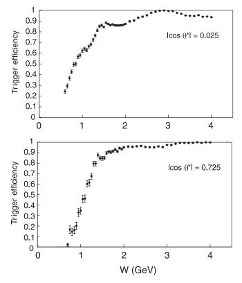
FIG. 6. Trigger efficiencies plotted as a function of W for two  $|\cos\theta^*|$  bins.
