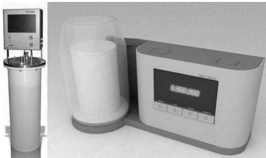
Fig. 1 Two cylindrical ionization chambers equipped with electronics. Active volumes are 11.8 L (left) and 1 L (right), respectively
