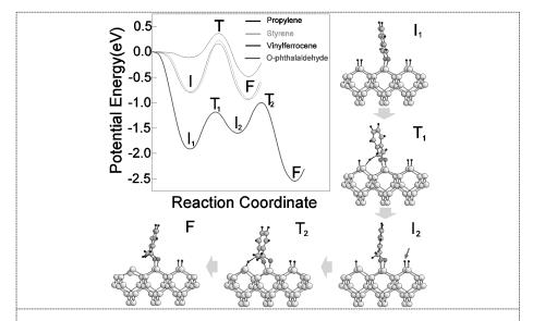
**Figure 1.** Calculated energy profile of H-atom abstraction for an adsorbed O-phthalaldehyde molecule on H-terminated Si(001) surface. The atomic geometries of the intermediate (I), transition (T), and final (F) states are given. The circles represent Si, C, O, and H atoms with decreasing size. For comparison, the energy profiles for propylene, styrene, and vinyl ferrocene are also given.
