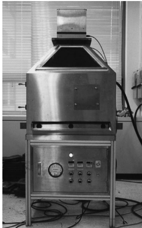
Fig. 2 Photo of fume collection chamber.
