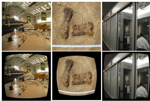
FIGURE 6. Fisheye image generation on real image (From the left, the values of k_1 are 0.0372, 0.1813, 0.0126; The values of k_2 are 0.0772, 0.1852, and 0.0432).
