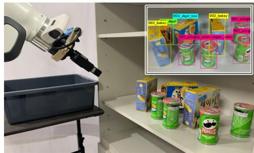
FIGURE 12. An instance of a real environment for experiments and a vision view from the vision sensor mounted on the wrist.
