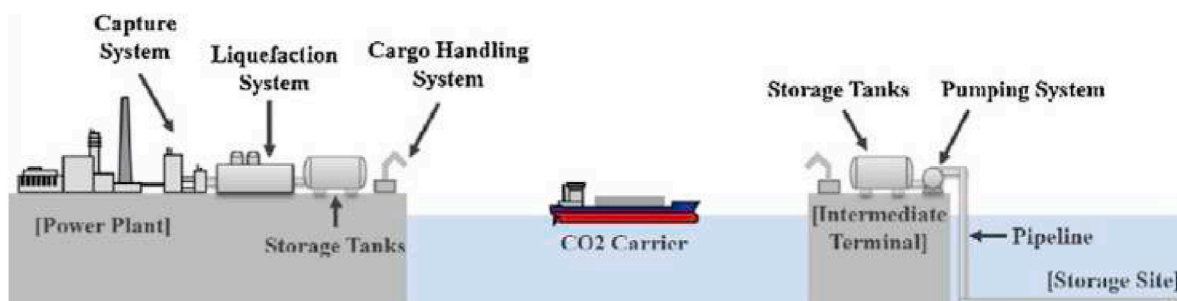
Fig. 25. The different modules involved in the CO 2 shipping process chain [64].
