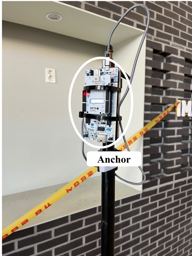
FIGURE 12. Installation of UWB anchors in experimental environment.
