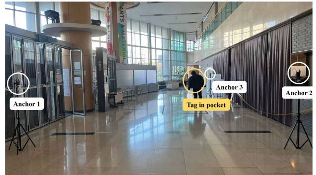
FIGURE 14. Indoor positioning experimental environment for tags in pocket.
