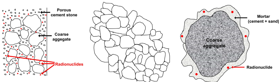
Fig. 1. Schematics of contaminated concrete, aggregate after recycling process of concrete and cross section of aggregate after recycling process of concrete.
