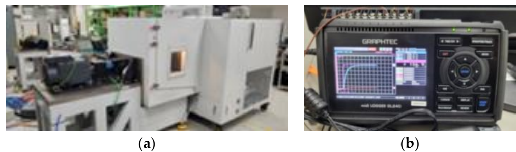
Figure 24. Experiment and measurement equipment for analyzing the change of back EMF due to temperature: (a) thermo-humidity chamber combined dynamo test bench; (b) temperature measurement using a temperature data logger.
