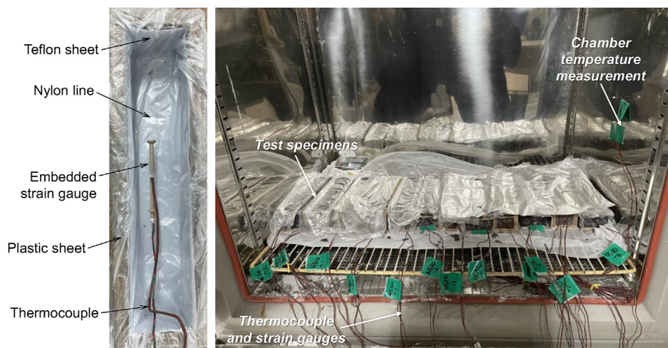
Fig. 4 – Test setup for autogenous shrinkage measurement.
