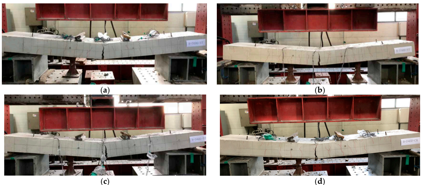
Figure 19. Flexural performance test failure pattern: (a) B-D200-ST; (b) B-D300-ST; (c) B-D400-ST; (d) B-D400-CR.
