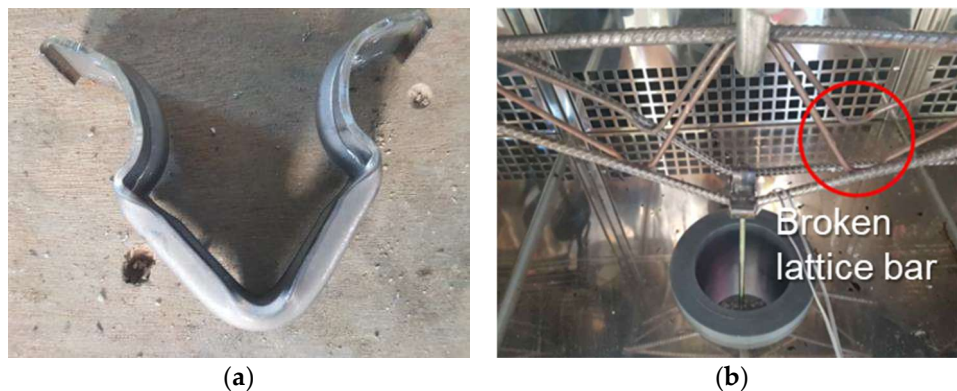
Figure 11. IR series failure shape: (a) IR-1.6T; (b) IR-2.0T.
