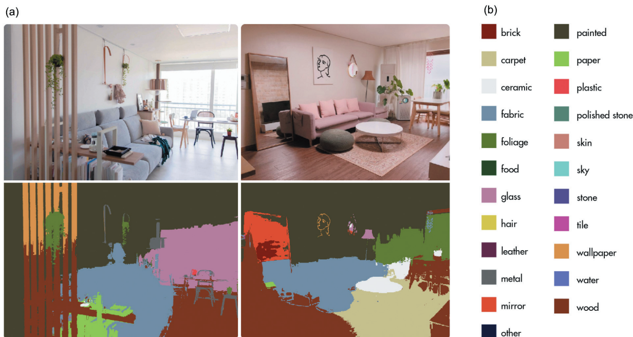
Figure 5: Material recognition and segmentation result. (a) Raw image and result image and (b) color by material area.
