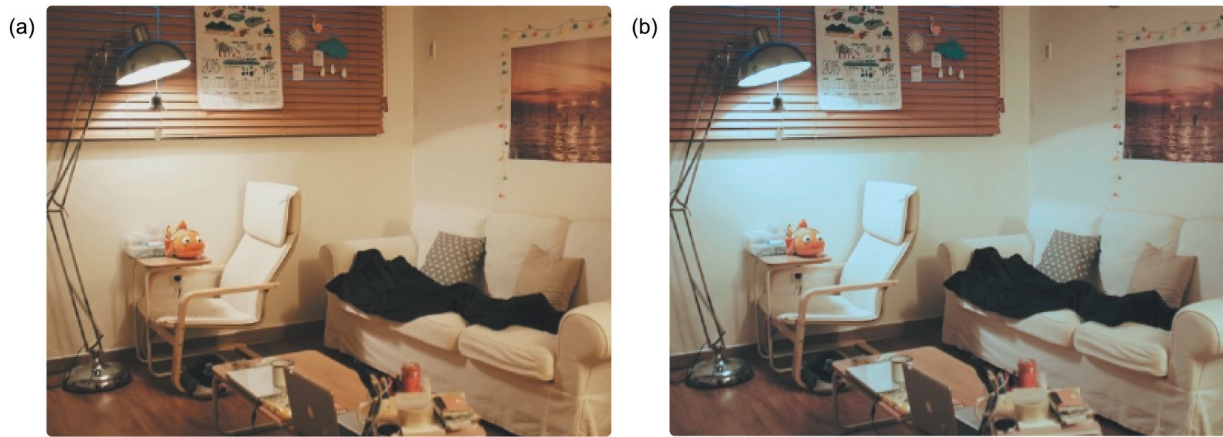
Figure 4: Image white balance example. (a) Raw image and (b) image with white balance process.
