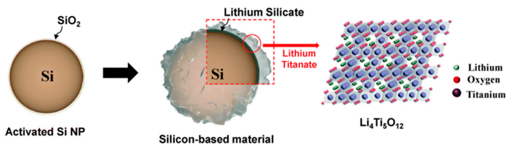
Figure 5. Schematic illustration showing the synthetic process of the Si-based multi-components. (Reprinted with permission from Ref. [47]. Copyright, 2015 Royal Society of Chemistry).
