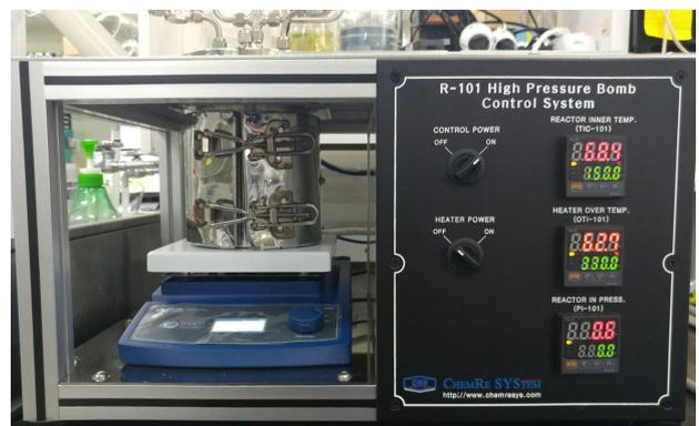
Fig. 1. A reactor designed to mimic an organosolv process.
