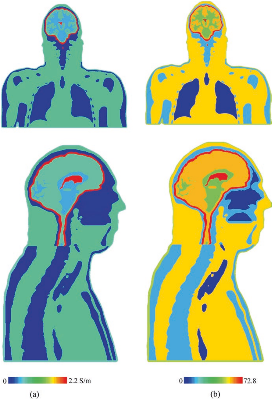
Fig. 13.10 Map of electrical properties for AustinMan model. (a) conductivity profiles (b) relative electrical constant profiles
