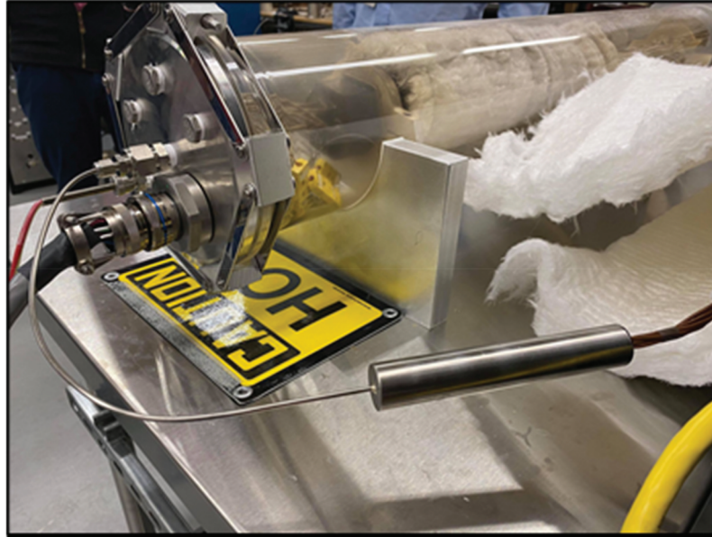
Fig. 17. Ten-point Type K thermocouple in SPHERE.
