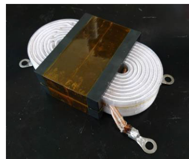
FIGURE 13. Planar transformer using the interleaved serpentine winding method.
