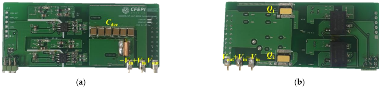
Figure 8. Photograph of the PCB with the proposed 3-D lattice structure. (a) Top view; (b) bottom view.
