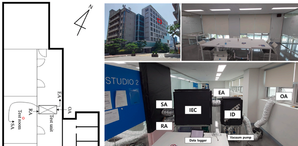
Fig. B.1. Experimental setup for simulation model validation of the proposed system.
