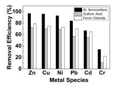
**Figure 1.** Metal removal efficiencies obtained by chemical (i.e., sulfuric or ferric chloride leaching) and bioleaching using *A. ferrooxidans*. The results were obtained at optimum operating conditions: pH, 2; pulp density, 2% (w/v); agitation speed, 120 rpm; and, temperature, 25 ± 2 °C. Data obtained from Bayat and Sari 2010 [22].
