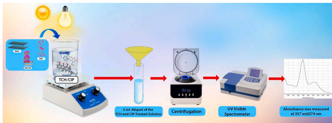
Scheme 2. Schematic representation of photocatalytic degradation studies of TCH and CIP.
