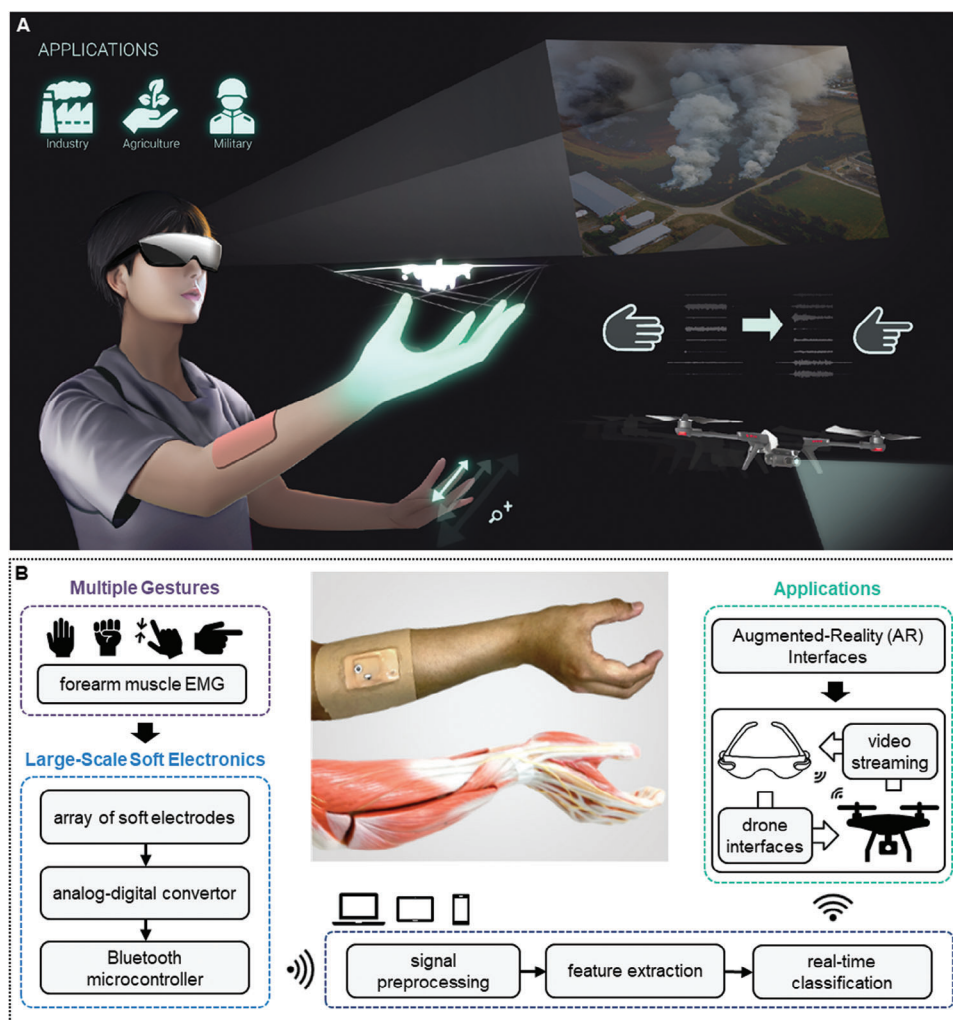
Figure 1. Overview of AR-enabled persistent human–machine interfaces via a scalable wireless soft electronic system. A) An illustration of a subject wearing an AR headset and a soft electronic patch for drone control via hand/wrist gestures. B) A flow chart describing the step-by-step process, including EMG-based gesture detection by using soft electronics, signal processing, data classification via machine learning, and real-time control of a drone with AR interfaces. The photo in the middle shows a close-up view of the soft electronic patch on the forearm and an illustration of forearm muscles where EMG signals are recorded through the device.
