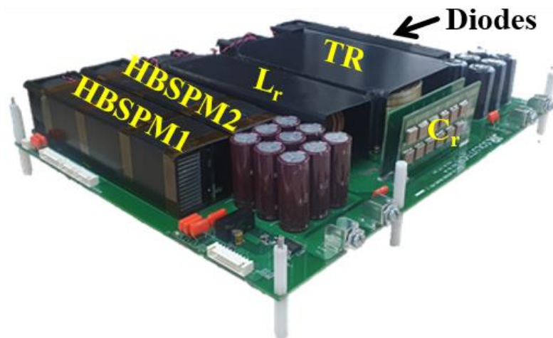
Figure 19. Full-bridge LLC resonant converter based on the proposed HBSPM.
