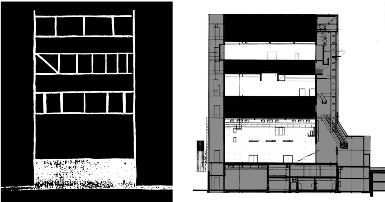
Figure 19. Solid and void elements at the ZKM: structural concept from Koolhaas' writing "last apples" (left) and an analysis of the building's section plan with indicated solid (black) and void (white) elements (right). Source: Koolhaas 1998b, 675 (left); Koolhaas 1998c, 89 (right; edited by author).
