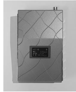
Fig. 1 Photo of a portable black carbon monitor
