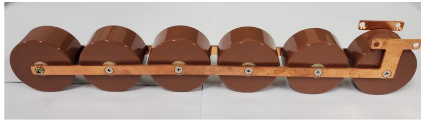
Figure 2. Picture of the six-stage PFN.
