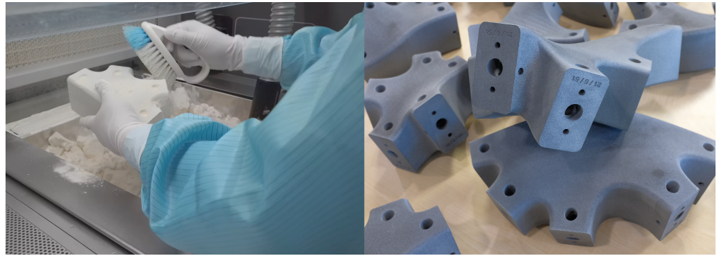
Figure 21. Post processing of 3D-printed parts and finished parts showing holes on each contact face for powder removal.
